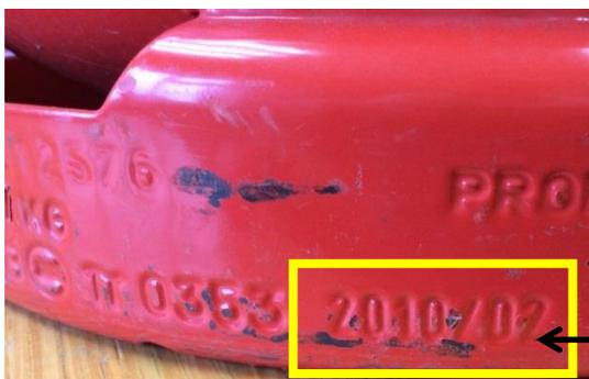
At the very bottom of the base ring the third row of text shows the date of manufacture i.e. 2008, 2009, 2010 or 2011.
